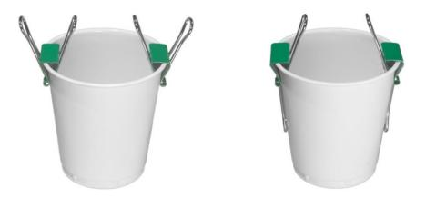
d. Place the second cup into the first so that the line joining its clips is at a 90-degree angle to the line joining the clips on the first cup.
