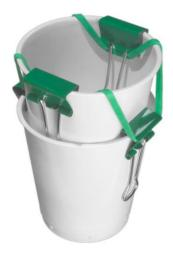
f. Turn the assembly over. Wrap one or two more rubber bands around the top cup to increase the visibility of the mine underwater and to generate more friction when a robot touches it.
