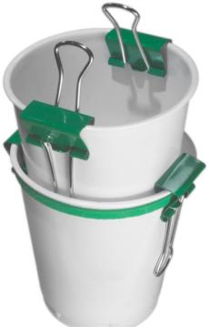
e. Pull each section of rubber band on the first cup up and over the handle of each clip on the second cup. Then flip the inner handles of the clips on the second cup down over the rubber band sections.
