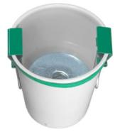
c. Get another 3-oz cup and clamp two small binder clips over the rim on opposite sides. Flip the outermost handles of the clips down. Leave the inner handles up.
